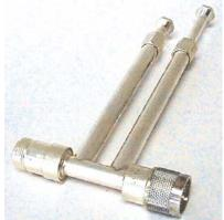
Microlab single, double and triple stub tuners are impedance matching instruments consisting of independently variable branch lines or stubs connected to a main line. A common application is in amplifier development to test operation under varying degrees of mismatch or load pull.
