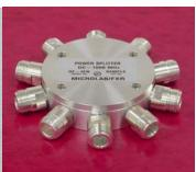
Microlab/FXR DA through DF series power dividers are miniaturized multi-terminal devices designed to separate or combine RF signals. They employ resistive elements to match one or more terminals to 50 ohms. Careful design of resistive elements and impedance matching techniques permit the use of these dividers at frequencies to 1.5 GHz.
